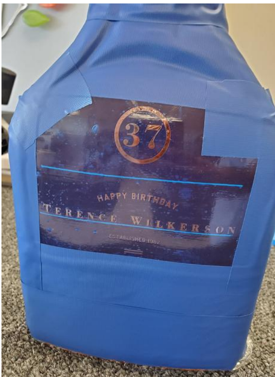
Vinyl Blasting Tape Applied
