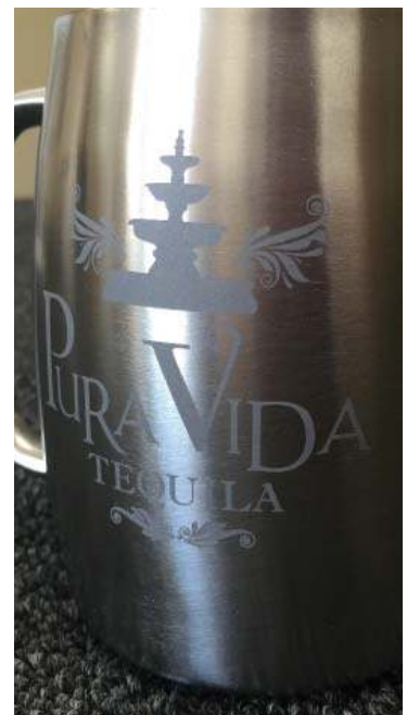
(above) Careful masking is imperative to ensuring clean lines when sandcarving or blasting metal items, and creates a template for any painting or color-filling to be done later.
