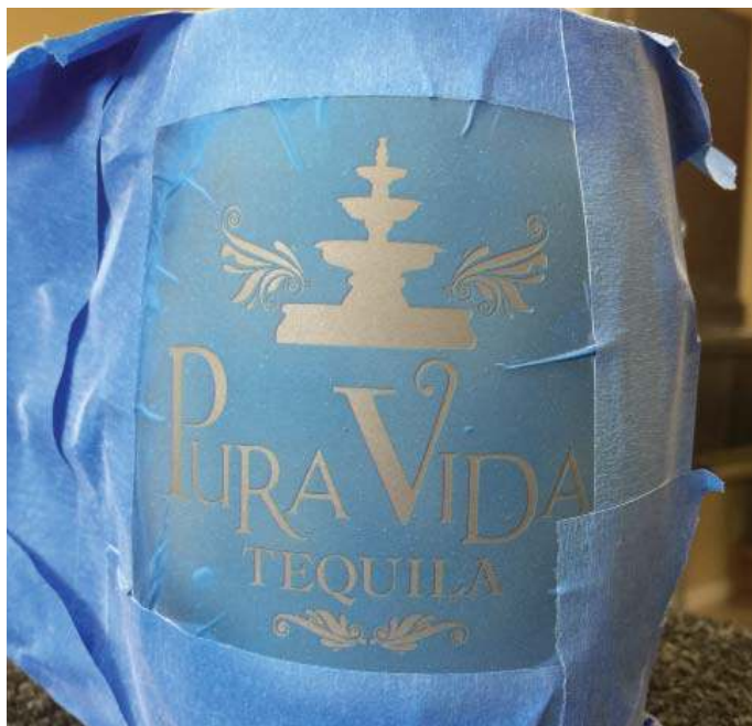
(above) Careful masking is imperative to ensuring clean lines when sandcarving or blasting metal items, and creates a template for any painting or color-filling to be done later.
